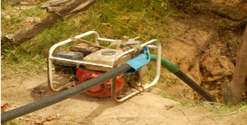
Plate 7: Pumping out water from tunnels during rainy season, Nandi County
