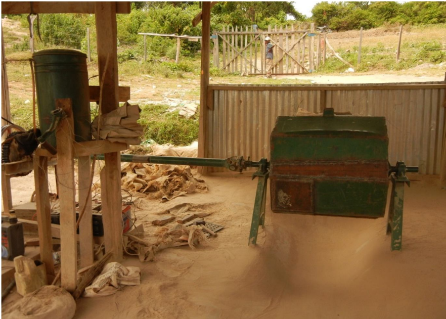
Plate 8: Fabricated Crushing machine in mining site, Nandi County
