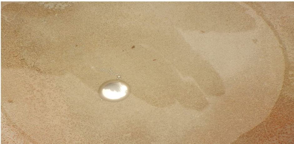
Plate 5: Use of mercury in amalgamation process, Nandi County
