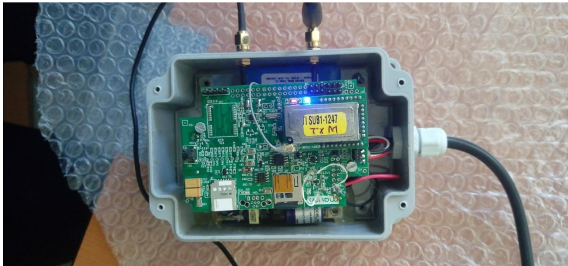
Figure 33 Gateway Router fitted with Zigbee Radio module and GSM gateway
