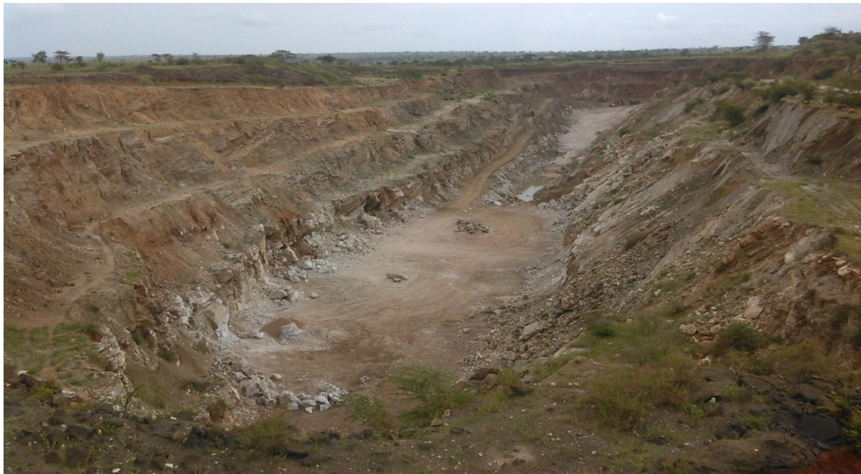
Figure 20: Benched Deep Open Cast Activities in the Study Area
