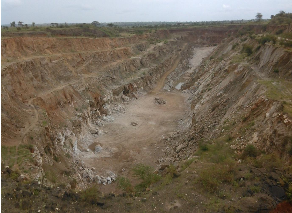
Figure 2: Benched Open Cast Mining Activities at Kibini Mine
